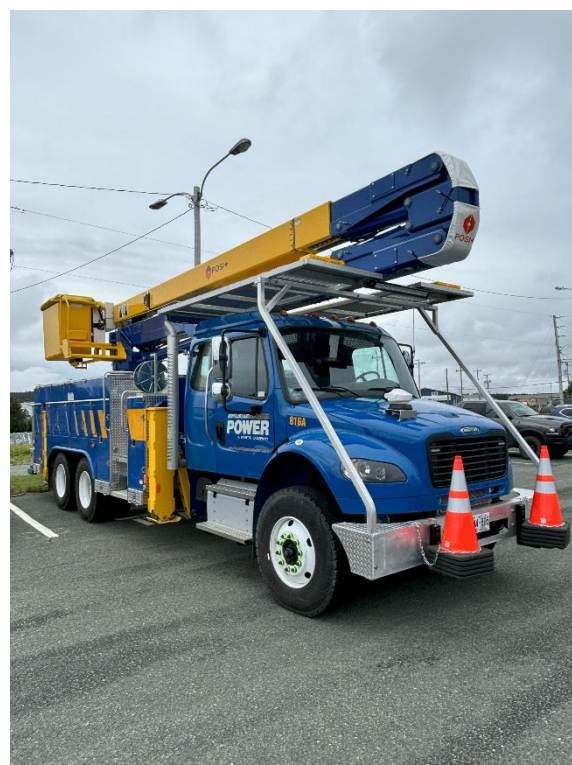
The first Newfoundland Power line truck outfitted with an electric power take-off that enables boom operation without running the truck engine.
